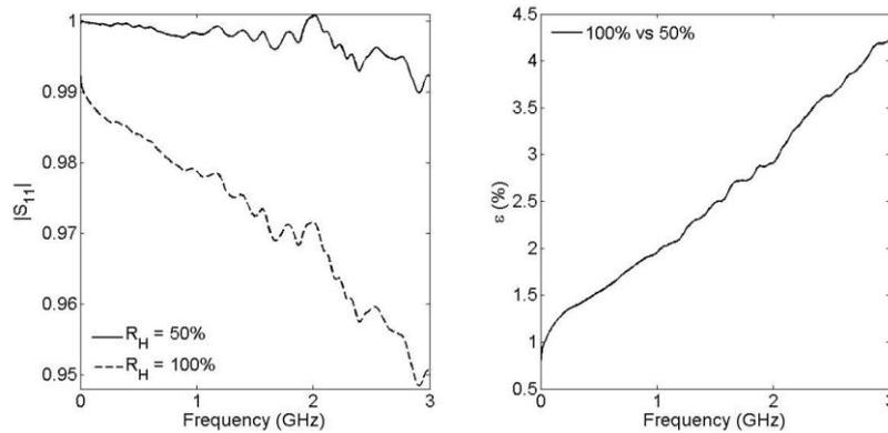
**Figure 2.** Measured probe  $|S_{11}|$  parameter for Hempcrete samples featuring 50% and 100%  $R_H$  respectively and relative absolute error  $\varepsilon = \left| \frac{|S_{11}^{R_H 100\%}| - |S_{11}^{R_H 50\%}|}{|S_{11}^{R_H 50\%}|} \right|$ .
