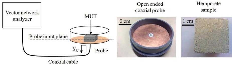
**Figure 1.** (a) Dielectric spectroscopy experimental set-up.
