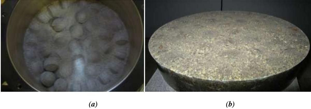
**Fig. 2:** (a) Bentonite mixture made up of pellets and powder, representative of the material at emplacement of nuclear waste repository seals ; (b) bentonite during the hydration phase.
